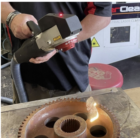
↑ LaserClean's hand held laser stripping rust from a metal surface (Source: LaserClean)
